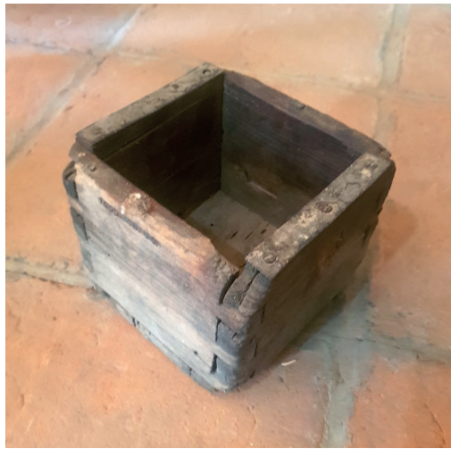
► Fig. 3. Photograph of a tlatamachihualoni dry measure now referred to as an almud . The almud volume is one liter and measures 10 cm x 10 cm x 10 cm (the Photograph is used with the permission of the Museo de Artesanías, Tlaxcala, Mexico).
